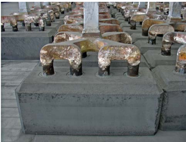
Fig 1: Pre-baked anode blocks rodded for high amperage pots are increasing in dimensions
