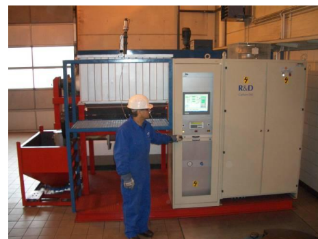
Figure 1. Length wise graphitization furnace for Ø50mm cores
