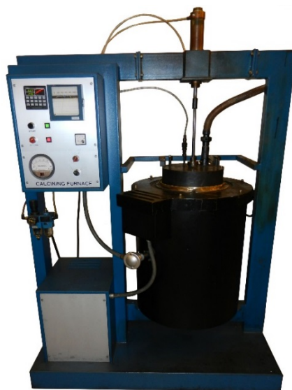
Figure 3: RDC 165 Söderberg baking furnace BF12S
