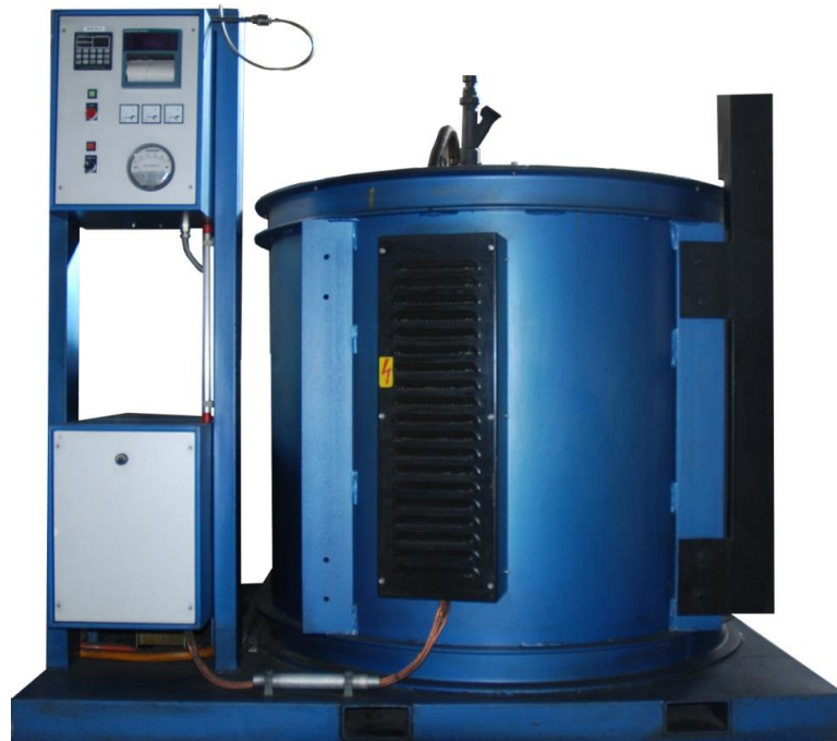
Figure 3: RDC 167 Pilot Baking Furnace BF24
