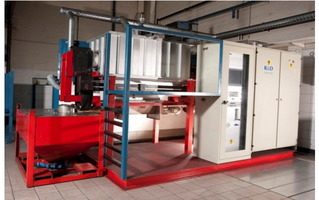
Figure 10: 80 kW LWG graphitizing furnace
