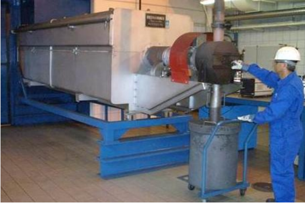
Figure 6: Rotary kiln (L=6m ø25cm) for coke calcinations
