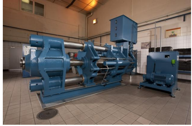
Figure 9: 400 tons extrusion press for 85mm green rods
