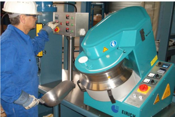
Figure 8: Intensive impeller mixer for high density paste (10 l)
