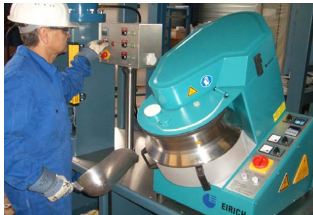
Figure 5 : Intensive impeller mixer for high density paste (10 l)
