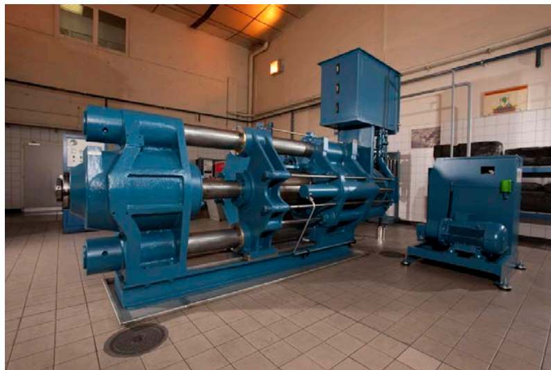
Figure 6: 400 tons extrusion press for 85 mm green rods
