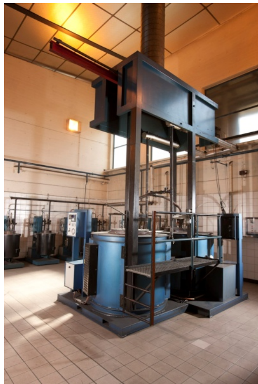
Figure 7: RDC 167 Pilot Baking Furnace BF24
