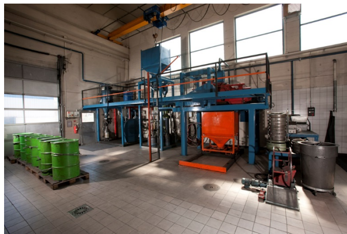
Figure 4: Pilot plant dry aggregate preparation
