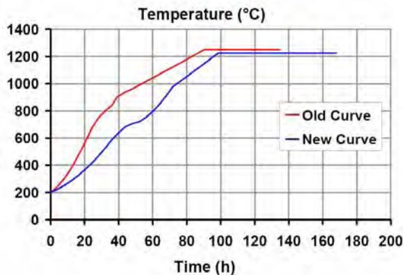
Figure 6. Target baking curve before and after the optimization
