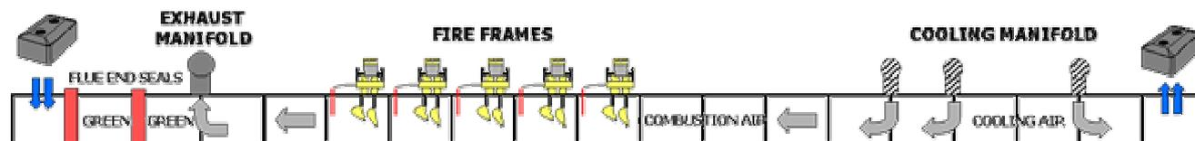
Figure 1. Original fire configuration prior to optimization with 2 pre-heating sections
