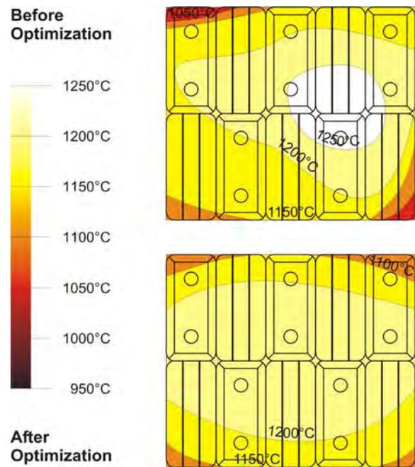
Figure 7. Final baking temperature distribution of anodes in the pits before and after the optimization
