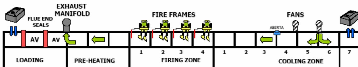
Figure 2. New fire configuration of furnace 1 after optimization
