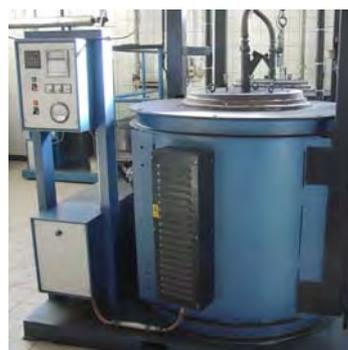
Figure 4. Baking of pilot electrodes
