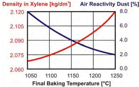
Figure 5. Influence of the final baking temperature on anode properties
