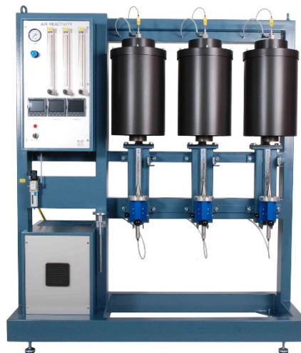
Figure 10: Test arrangement for the determination of the air reactivity
