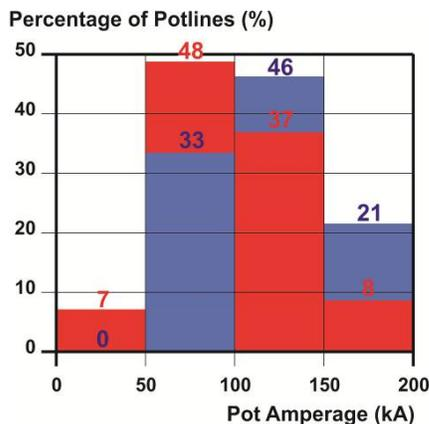
Figure 1: Line current, 1990 vs. 2013 1990 in red, 2013 in blue
