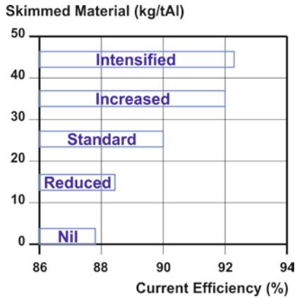
Figure 3: Skimming and current efficiency
