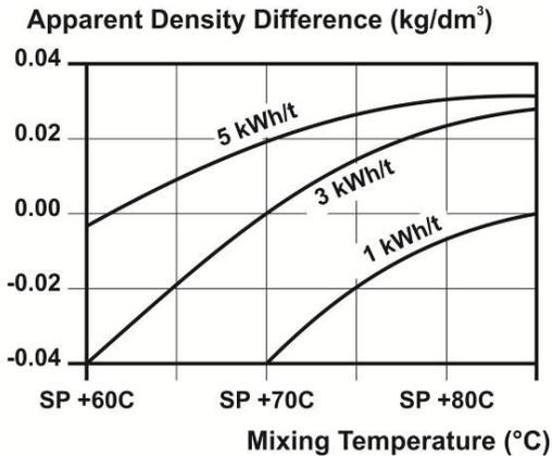
Figure 11: Impact of kneading temperature and energy
