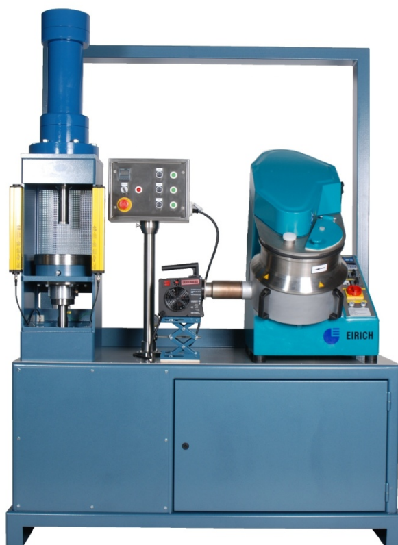
Figure 3: RDC 161 Bench Scale Anode Production Unit
