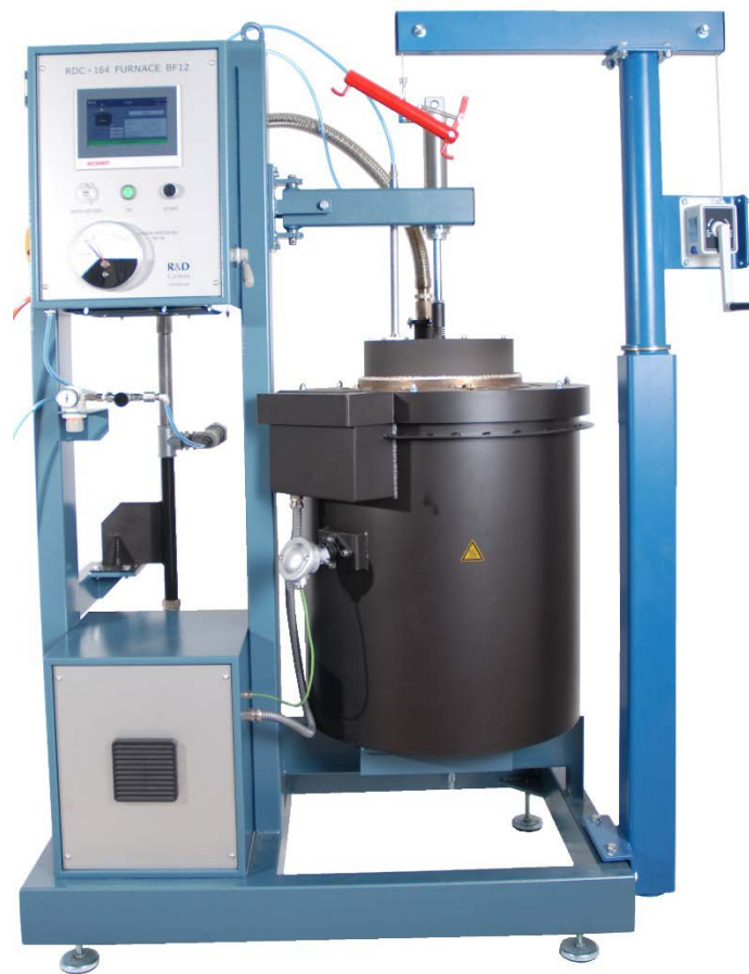
Figure 2: RDC 164 Calcining Furnace BF12 C
