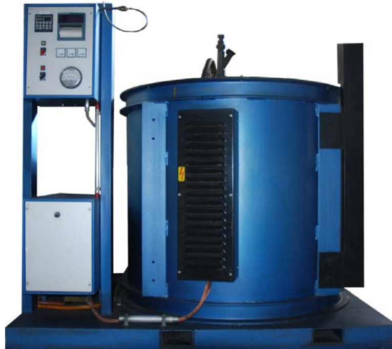
Figure 4: RDC 167 Pilot Baking Furnace BF24
