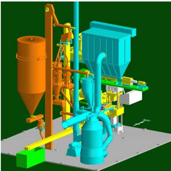
Fig 4: Equipment arrangement in a 600'000 t/y paste plant
