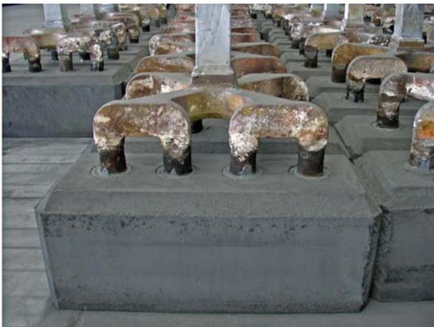
**Fig 1: Pre-baked anode blocks rodded for high amperage pots are increasing in dimensions**
